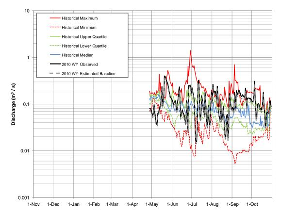
Note: Observed 2010 WY hydrograph based on Station S12, Fort Creek at Highway 63, 2010 WY provisional data from April 27 to October 30. The upstream drainage area is 31.9 km<sup>2</sup>. Historical values from April 27 to October 30, 2010 were calculated using data collected from 2000 to 2002 and from 2006 to 2009.
