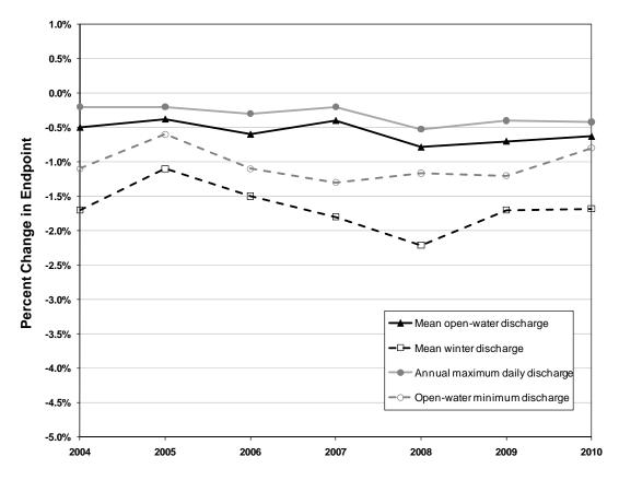
Note: Measurement endpoints are calculated from estimated *baseline* and observed *test* hydrographs at Station S24, Athabasca River below Eymundson Creek.
