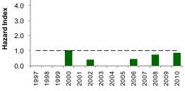
\* Total metals include: As, Ba, Be, Cd, Cr, Co, Cu, Pb, Hg, Mo, Ni, Se, St, Th, Ti, Sn, Ag, U, V, Zn (measured in all years). \*\* Dashed line indicates potential chronic effects level (HI = 1.0)
